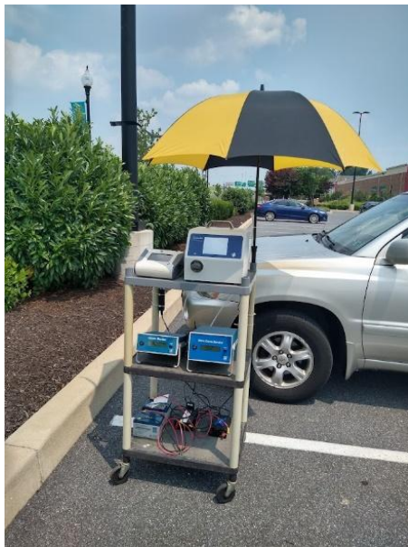
Fig. 1 From Left to Right, Top to Bottom: TSI Optical Particle Sizer, TSI Scanning Mobility Particle Sizer, 2B Technologies Ozone Monitor, 2B Technologies Nitric Oxide Monitor (discontinued use after Lancaster)
