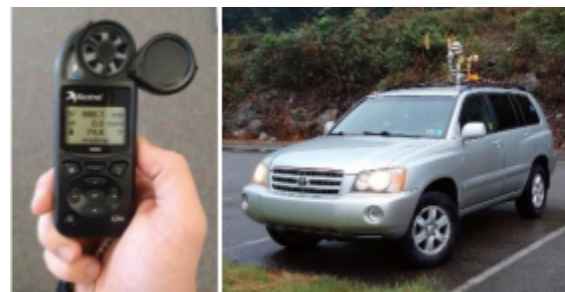
Fig. 2 Left: Kestrel 5000 Handheld Environmental Meter Right: Modified TWI WLS 8000 mounted on a vehicle
